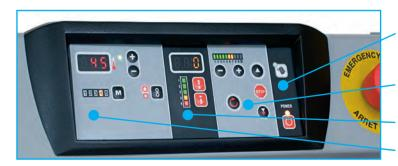
Foot switch selection and power button (when switching the machine off, the upper roller automatically lifts up in order to preserve the rollers).
